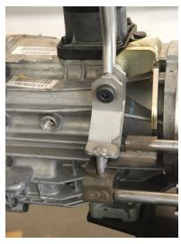
J-shift twin stick shown installed on AA bracket.
